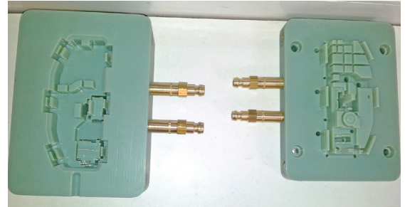
Figure 9: Cooling line connections on PolyJet core and cavity.
