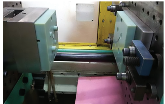
Figure 10: PolyJet mold without ejection system attached to steel backing plates.
