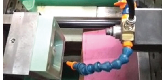
Figure 32: Cooling fixture for blowing air onto the PolyJet mold.
