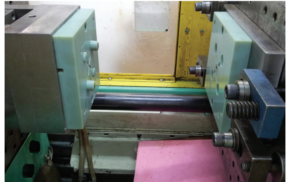
Figure 25: Attach core and cavity to steel plates and modular ejection system.
