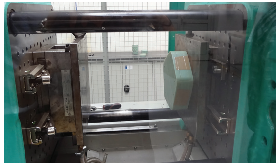
Figure 26: Assemble mold and attach to steel plate with double-sided tape.
