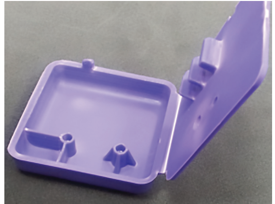
Spec resin provides functional testing of the living hinge.
